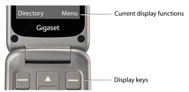
▶ Press the display key . . . The function shown in the display above is called, e.g.:
